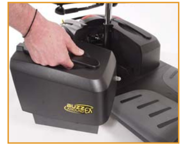
Step 2: Pull out the battery pack!
