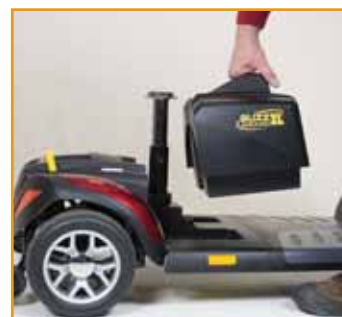
Step 2: Pull out the battery pack!
