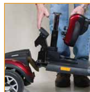
Step 4: Pull forward on the drivetrain release lever to separate the front and rear frame sections!
